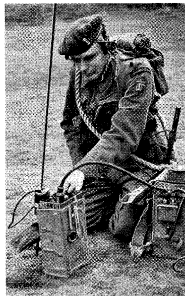
The No. 46 set unpacked for stationary operation with a heavy type of aerial. The case on the right contains the two batteries.
